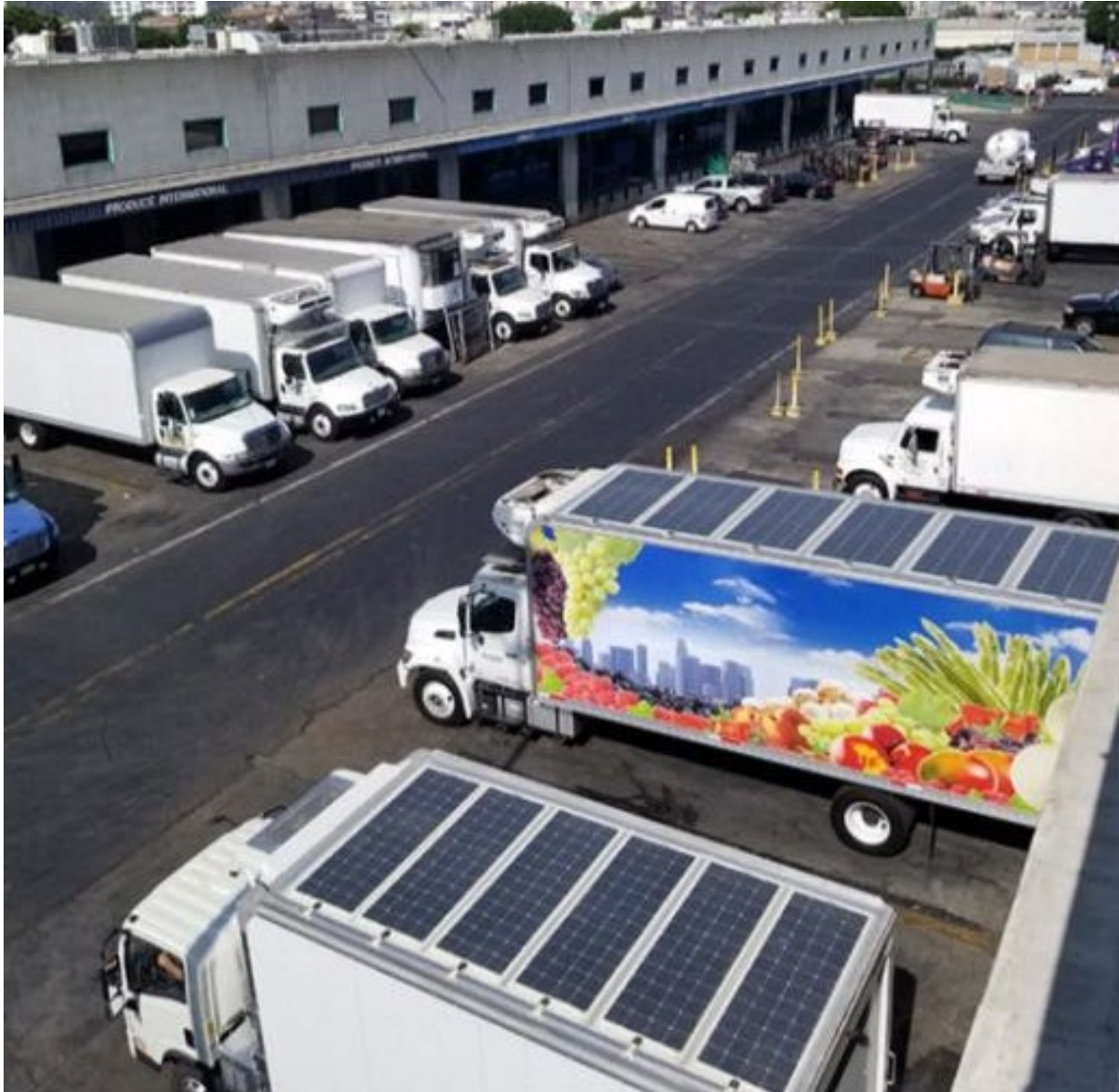
Figure IX-1. Battery-Electric Truck TRUs with Solar Assist
